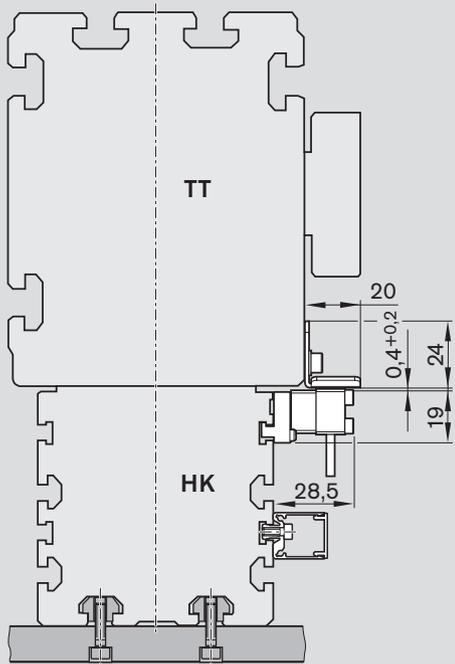
Proximity switches with attachments / cable duct
