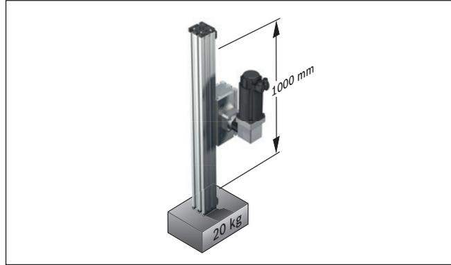
$$\begin{aligned} \text{Excess travel: } s_e &= s_{\max} + L_{ca} + L_{ad} \\ &= 2 \cdot u = 2 \cdot 31.88 = 63.76 = 64 \text{ mm} \\ \text{Max. travel distance: } s_{\max} &= s_{\text{eff}} + 2 \cdot s_e \\ &= 1\,000 + 2 \cdot 64 = 1\,128 \text{ mm} \\ \text{Module length: } L &= 1\,128 + 260 + 130 = 1\,518 \text{ mm} \end{aligned}$$
