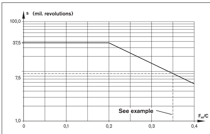
**Conversion of lubrication interval s from millions of revolutions to kilometers:**
