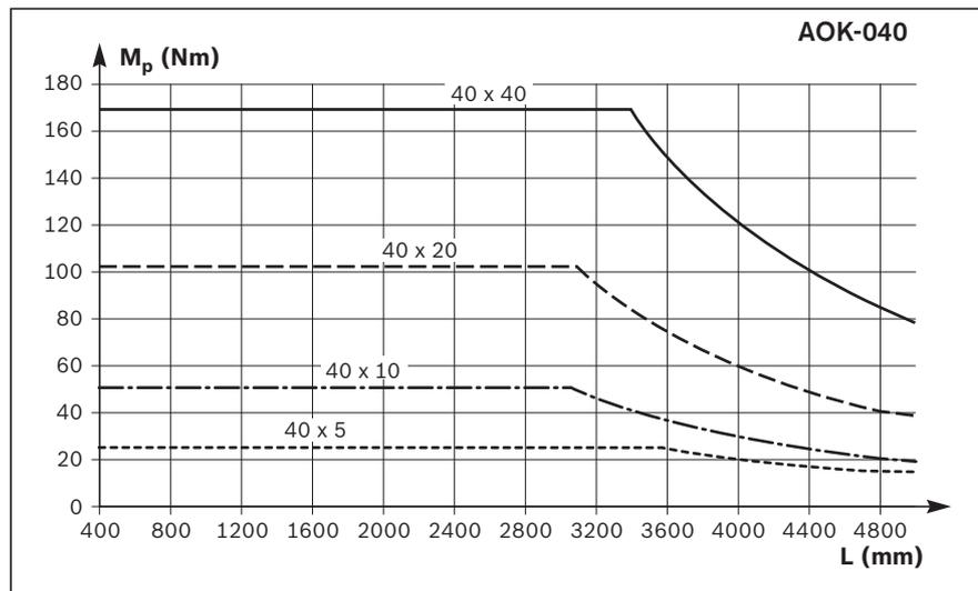
**Permissible drive torque  $M_p$  with fixed bearing only**
