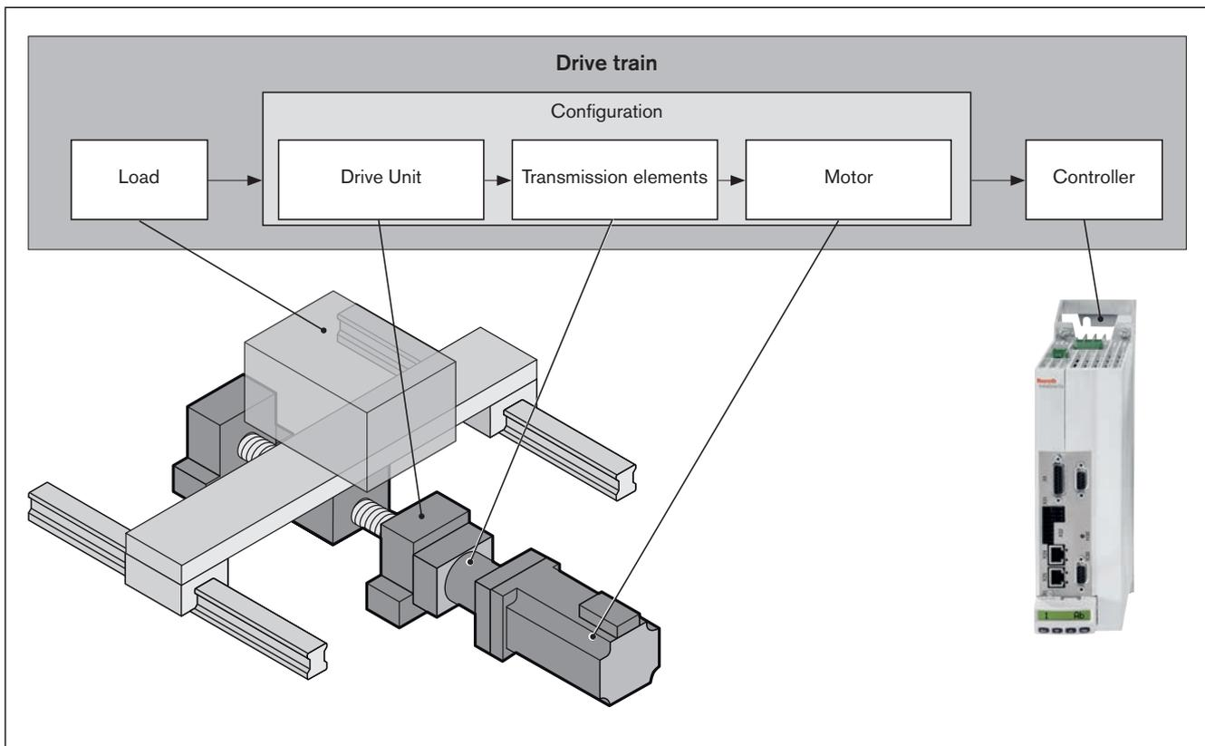
Correct dimensioning and assessment for an application requires structured consideration of the entire drive train. The basic element of the drive train is the configuration comprising the Drive Unit, the transmission element (coupling or timing belt side drive) and the motor, which can be ordered in this constellation as per the catalog.
