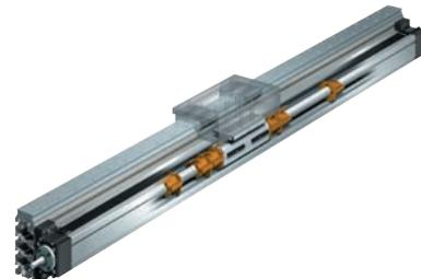
The table is supported symmetrically on two rail guides with four Runner Blocks. The Nut Housing of the ball screw drive is located at the top.
