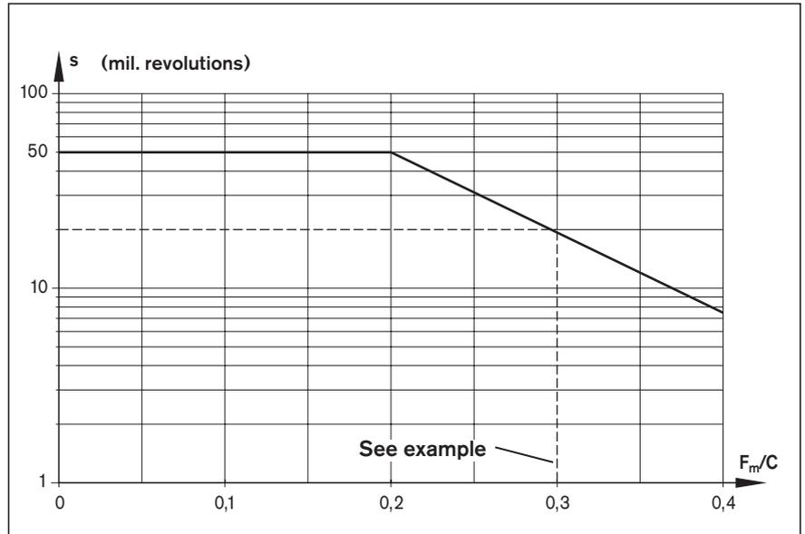
**Conversion of lubrication interval s from millions of revolutions to kilometers:**
