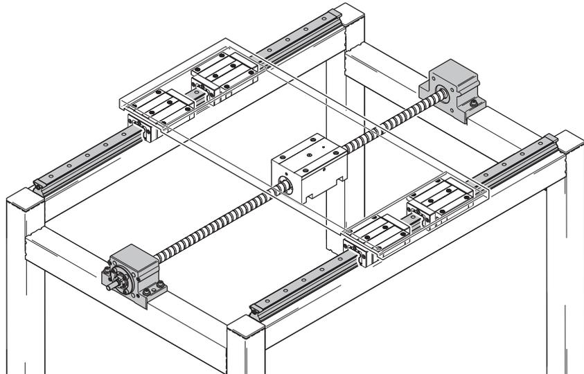
In this example, two separate linear guides, each with two Runner Blocks, absorb forces and torques so that when moving the structure only axial forces act on the Drive Unit (here AGK).
