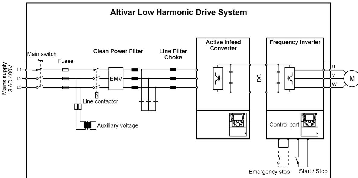
The modular construction makes it possible to adapt it to the individual requests. This makes the planning easy and helps to ensure a quick installation and commissioning of the drive.
