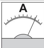
This option indicates the line current. It includes a measuring instrument built-in into the enclosure door and a current transformer.
