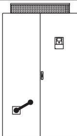
The main switch is able to switch the supply voltage of the frequency inverter. The external door handle enables handling of the switch without opening the enclosure door.
