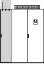
This option allows the connection of the mains and motor cables from the top of the enclosure.
