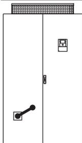
The external door handle enables handling of the switch without opening the enclosure door.
