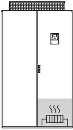
This option is used to heat the enclosure in order to avoid frost and condensation up to an ambient temperature of  $-10^{\circ}\text{C}$ . It includes the enclosure heating, a thermostat and a circuit breaker. The option is wired to the customer terminals X04 (max. cable cross section:  $4\text{ mm}^2$ ).
