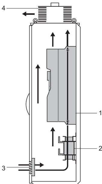
At protection degree IP54 with filter mats the input of the cooling air takes place through the filter mats in the enclosure door and the output through the fan at the top of the enclosure.
