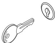
This option includes a key switch built-in the enclosure door, which switches between remote mode (terminals or bus) and panel mode. The panel control of the device occurs by means of the keys on the built-in LED-keypad or the removable operation panel, which is also built-in the enclosure door.
