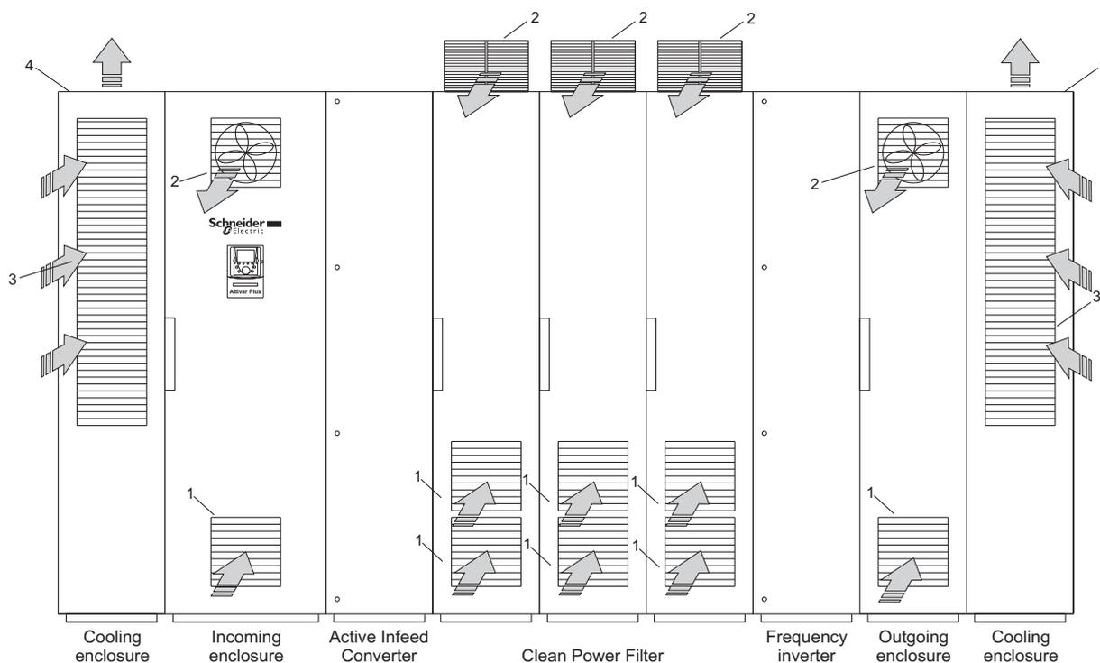
In case of this enclosure design the cooling of the power part takes place in an own enclosure. Here the cooling air is sucked in by the fans in the enclosure door and the air outlet takes place through the enclosure roof. The control part is cooled by fans in the enclosure door. At the Clean Power Filter the input of the cooling air takes place through the filters in the enclosure door and the output through the fans at the top of the enclosure.
