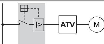
The circuit breaker is built-in instead of the main switch. It provides a switching-off at overload.
