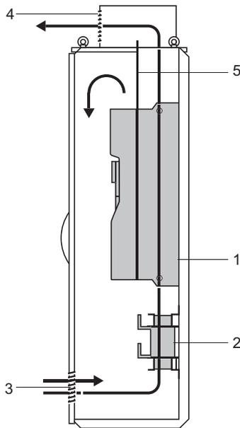
In this case the input of the cooling air takes place by the enclosure door and the output through the top of the enclosure. The fan of the power part, which is inside the device, provides the exhaust of the enclosure.
