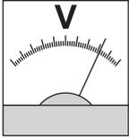
This option indicates the line voltage. It includes a measuring instrument built-in into the enclosure door and a phase selection switch.
