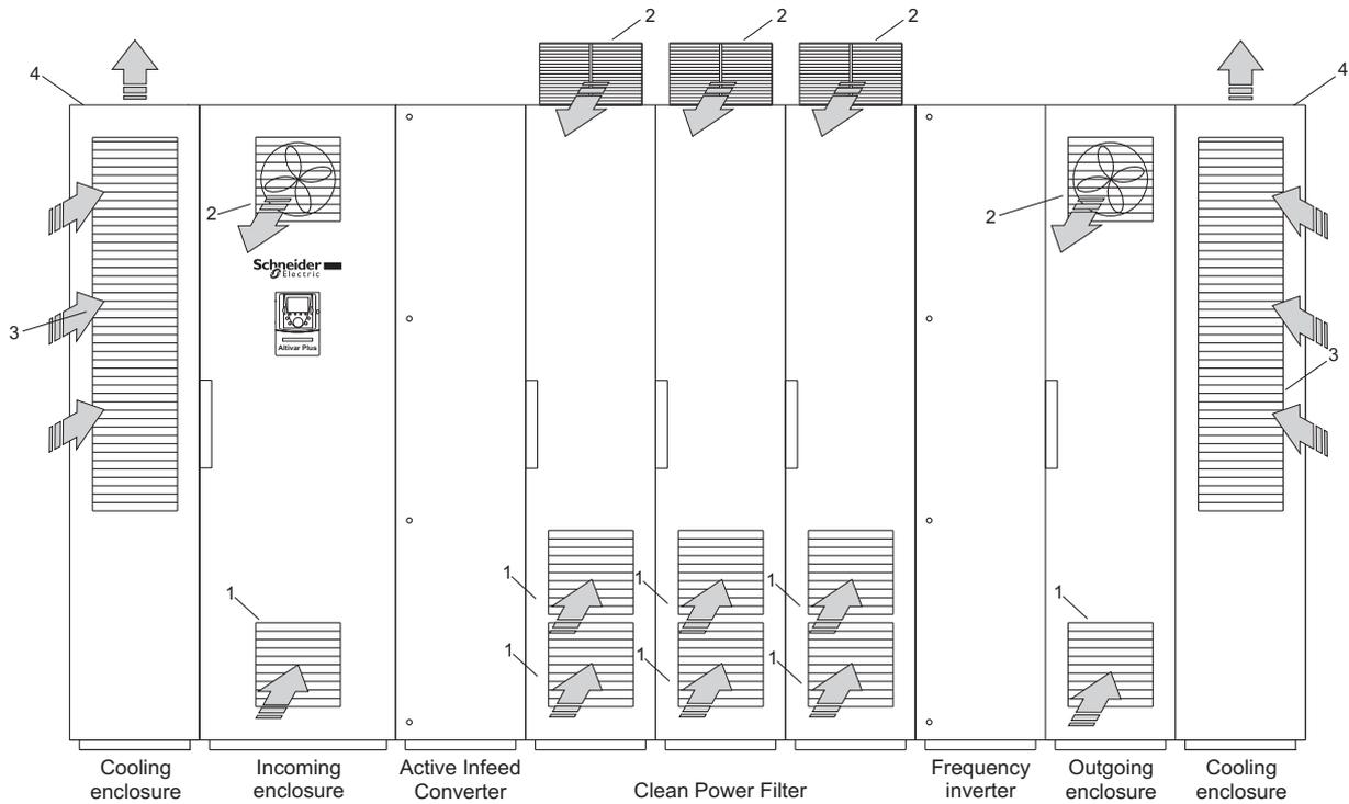
In case of this enclosure design the cooling of the power part takes place in an own enclosure. Here the cooling air is sucked in by the fans in the enclosure door and the air outlet takes place through the enclosure roof. The control part is cooled by fans in the enclosure door. At the Clean Power Filter the input of the cooling air takes place through the filters in the enclosure door and the output through the filter fans at the top of the enclosure.
